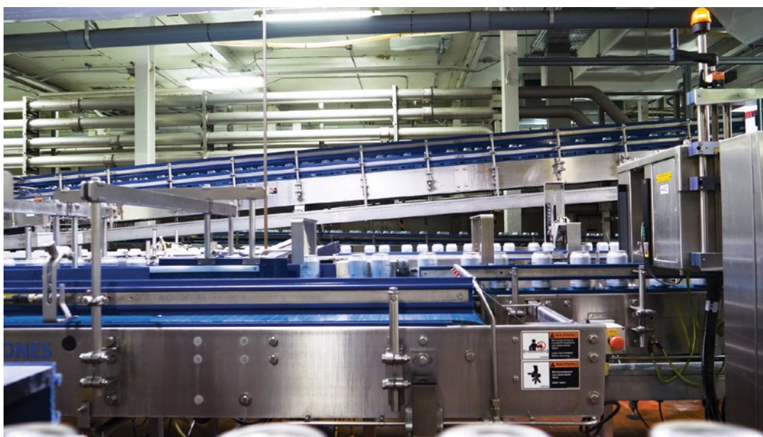
Capable of reaching throughput speeds of up to 300 containers per minute, depending on container type and style, the Performance case-packers patented Intelligent Synchronization technology allows it to control and monitor product flow and accumulation without the use of any mechanical devices.
