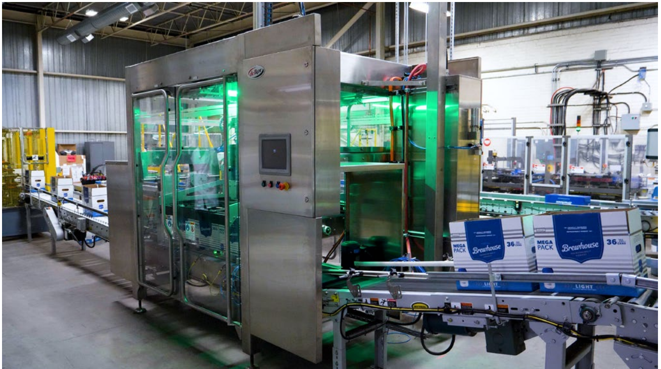
Right: The Performance series case-packer from Delkor Systems has been dedicated to the case-packing of large-format Mega Pack beer cases holding 36 or 48 cans of beer per case.
